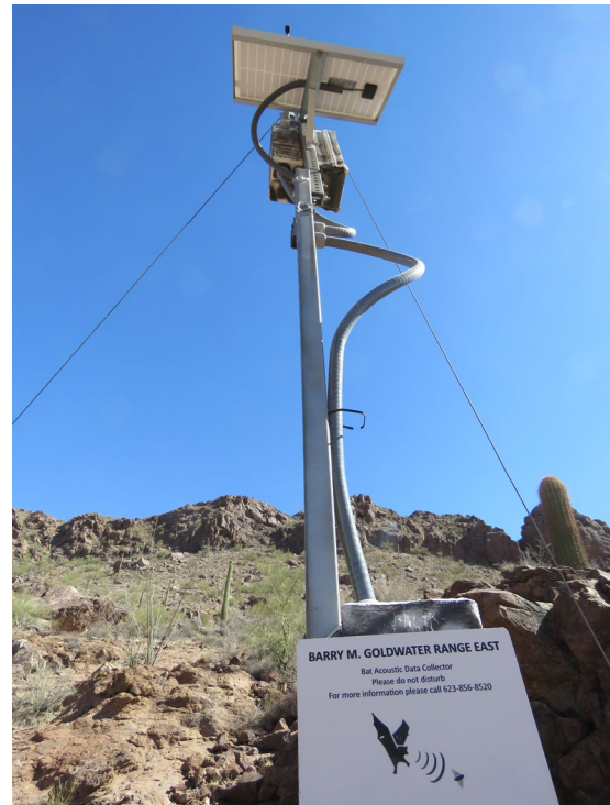
Bat acoustic monitoring devices provide continual monitoring of bats with minimal disturbance.
